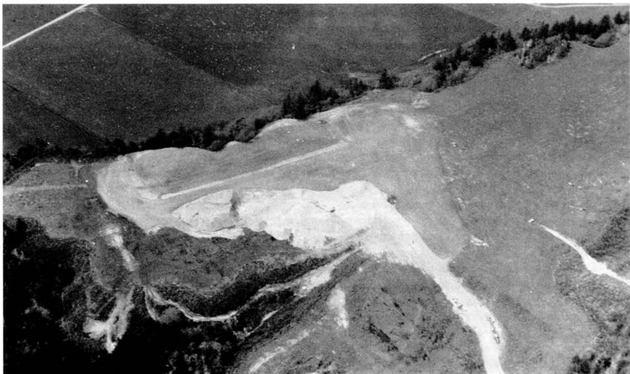
Figure 12. Rock-material site 334 after it has been shaped and seeded. Only stockpile area is unreclaimed.
