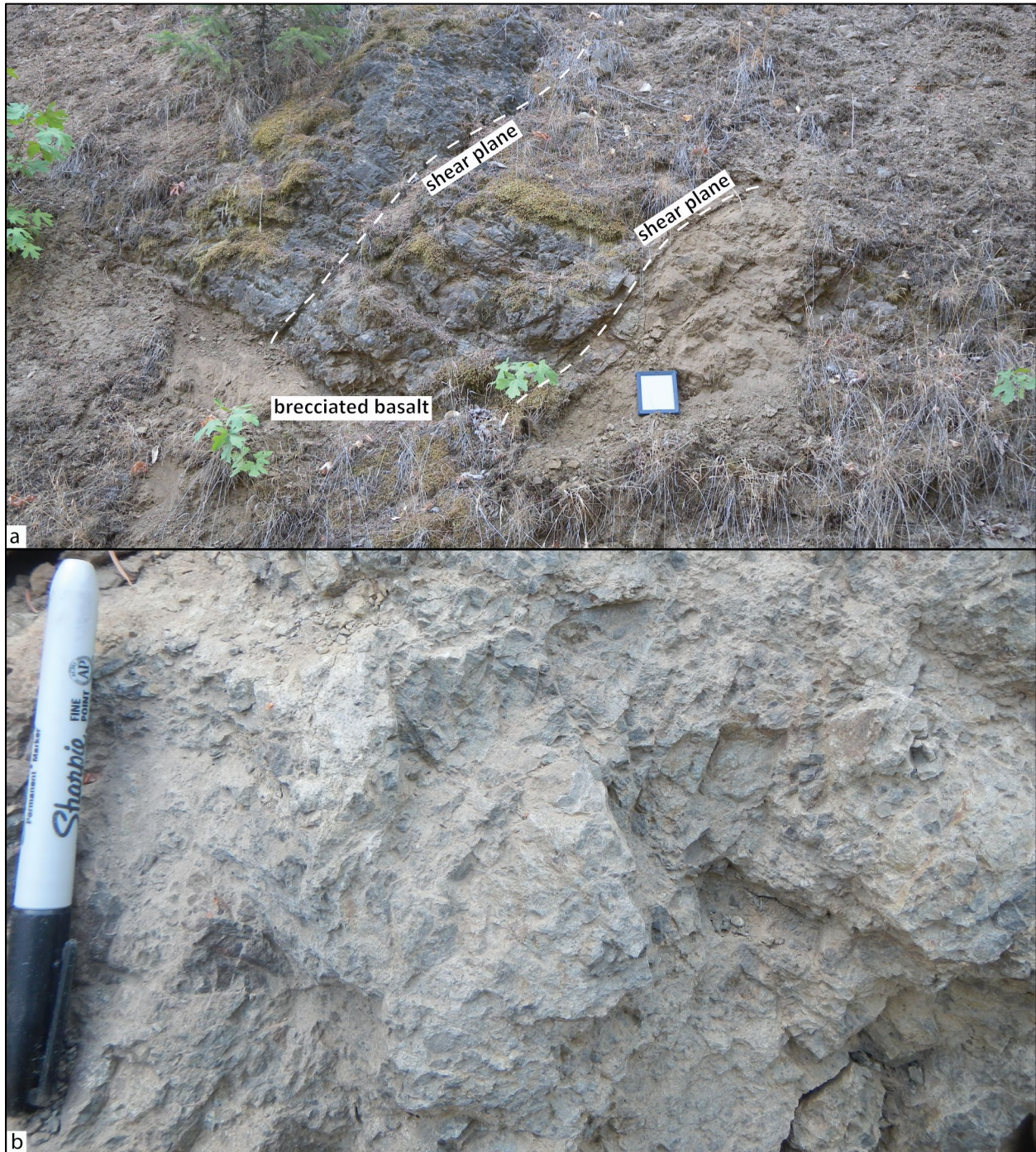
Figure 6-82. Fault breccia (QTfb) cropping out along North Fork Mill Creek. (a) QTfb in outcrop (45.53379, -121.40251). The iPad for scale is 25 cm (10 in) tall. View is looking southeast. (b) Closer view of QTfb from the outcrop in (a). Pen for scale is 15 cm (6 in) long. Photo credits: Jason McClaughry, 2015.
