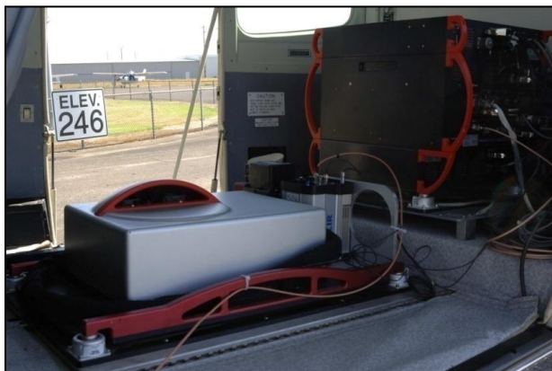
Figure 2. Pictures above are WSI's FLIR SC6000 integrated with a Leica ALS50-Phase II LiDAR System installed in one of WSI's Cessana Caravans. The SC6000 utilizes the same GPS/IMU system as the LiDAR system for direct computation of image external orientation
