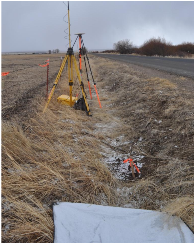
Figure 7. GPS base station set up with “space” blanket target set up near the control monument. The space blanket has a very low emissivity compared to the surrounding terrain and is detectable in the TIR imagery. The blankets were paired with small, catalytic heaters to quantify the accuracy of the TIR mosaic
