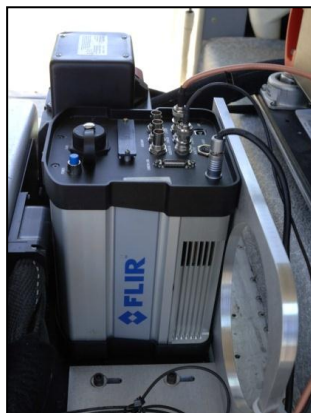
Figure 2. Pictures above are WSI's FLIR SC6000 integrated with a Leica ALS50-Phase II LiDAR System installed in one of WSI's Cessana Caravans. The SC6000 utilizes the same GPS/IMU system as the LiDAR system for direct computation of image external orientation
