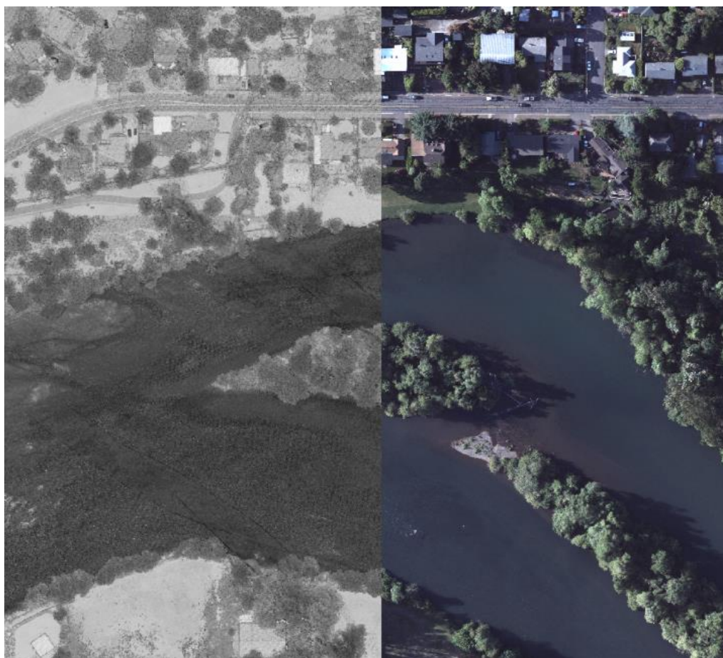
Figure 23: Image displaying the co-registration between the LiDAR intensity image and the orthophoto at a location within the Willamette River Topobathymetric LiDAR site.
