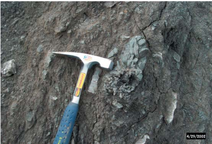
Figure 11. Sheared Jurassic mudstone and sandstone typical of the lower part of many bluffs in the study area. This material has little resistance to wave erosion or slope failure when it is as highly sheared as in this example. Shears are in so many different directions that bluffs are highly vulnerable to slope failure from rotational and translational landslides or block falls.
