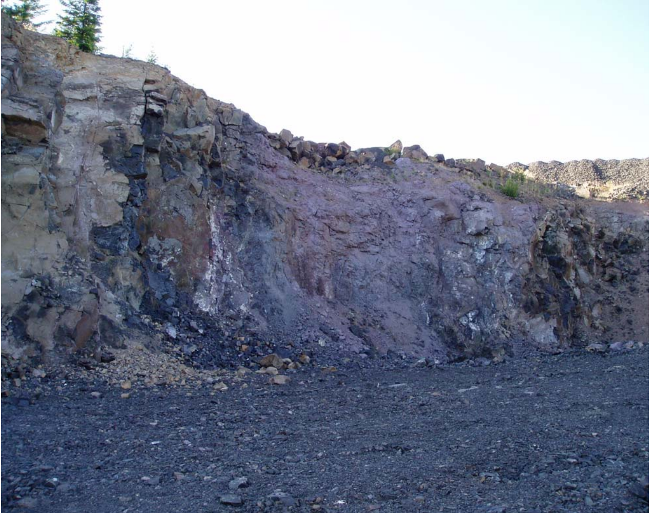
Figure 8. Quarry exposures of fresh black basalt (on left) with 100 ft (30 m) wide vertical walled zone of purple-gray hydrothermally altered basalt.
