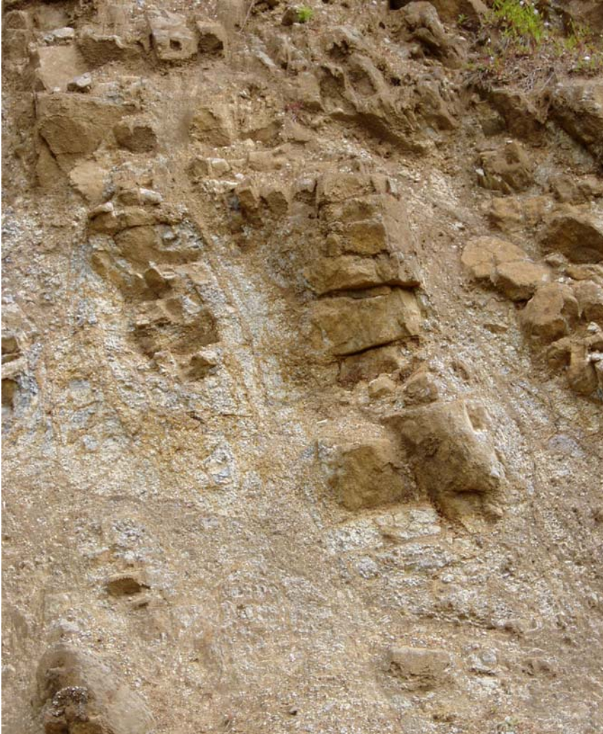
Figure 6. Severely weathered or hydrothermally altered blocky jointed basalt.
