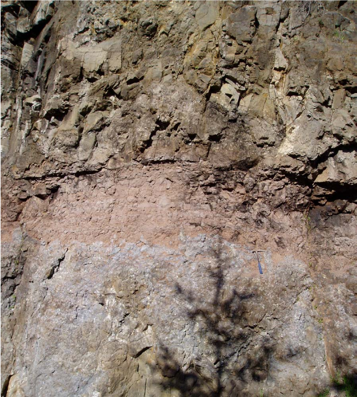
Figure 7. Contact between two basalt flows. Upper blocky jointed flow is relatively fresh, underlying flow has rubbly vesicular top that is soft, altered to clay voids filled with zeolites, overlain by about 1m of red basalt completely altered to clay with relict olivine and pyroxene phenocrysts visible.
