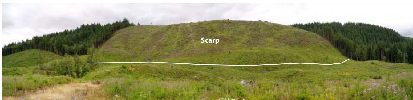
Figure 4. Part of the Wildwood landslide complex head scarp. Panoramic view looking west from station PDX-900 (NAD 83 UTM coordinates 507,214 m E, 5,059,187 m N). Clear-cut area of scarp is 500 m wide; scarp is 80 to 90 m high. Note chaotic terrain in foreground.
