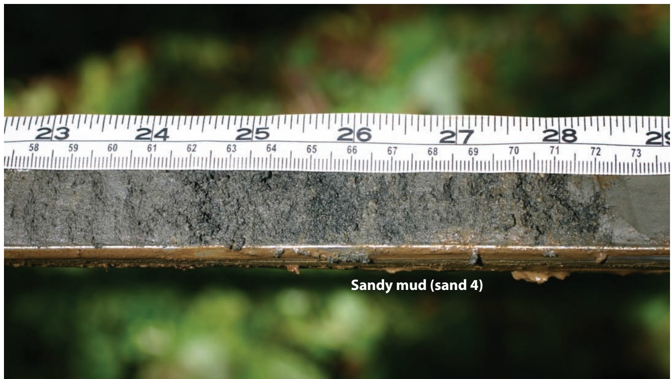
Figure 16. In contrast to the other sand layers in the Ecola Creek valley, sand layer 4 (core 73) consists of sandy mud with abundant volcanic rock fragments derived from the creek channel. Scale is in inches (top) and centimeters (bottom). Top of core is to the left.
