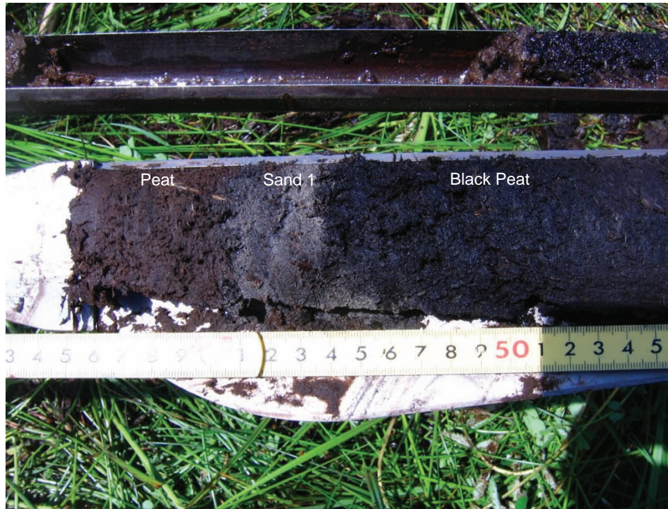
Figure 10. Quartz-rich, fine-grained, well-sorted sand characterizes sand layer 1 in Pompey Marsh. Scale is in centimeters. Top of core is to the right of the photo.
