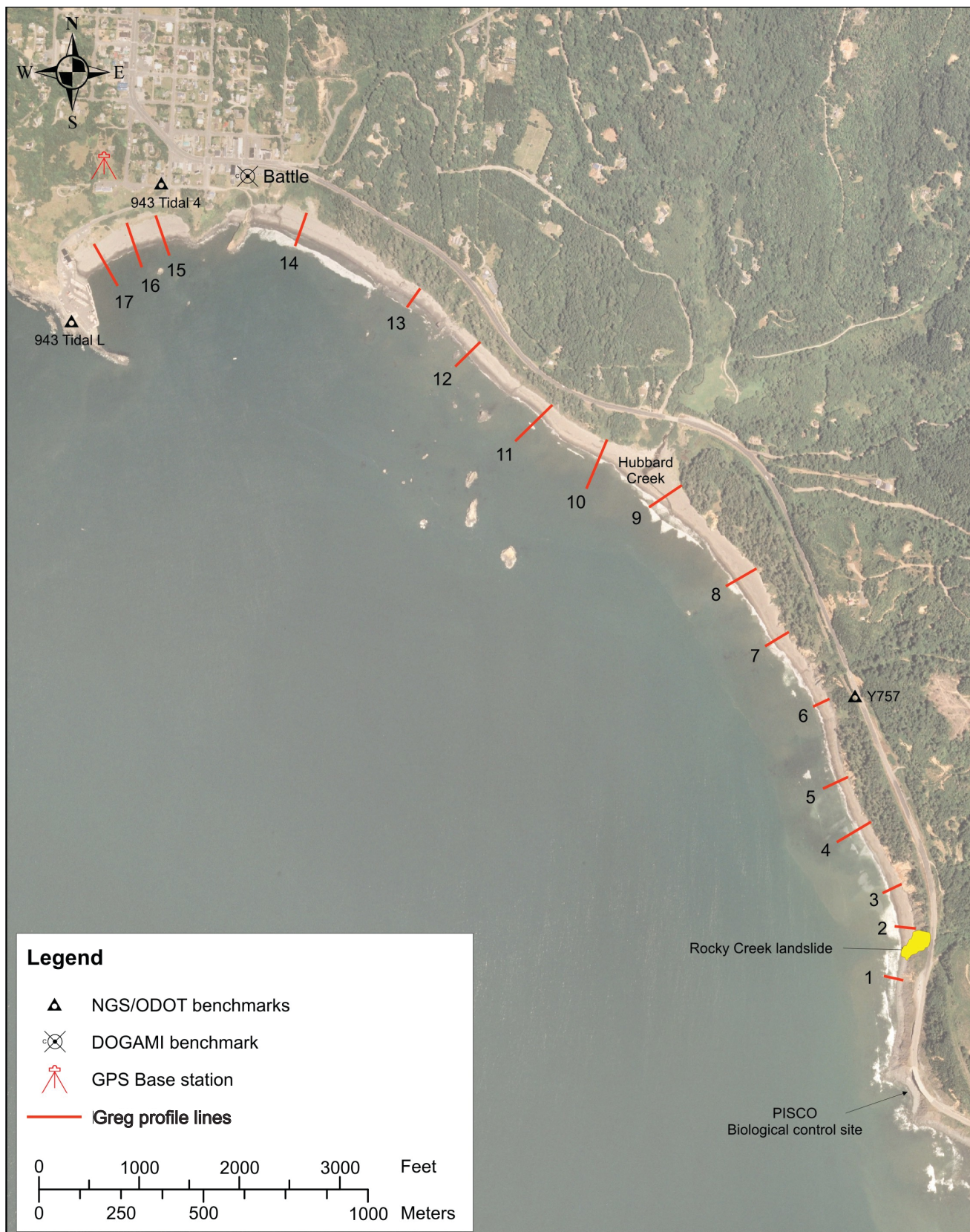
Figure 3. Location map showing the distribution of beach profile stations established in the Hubbard Creek littoral cell, Global Positioning System (GPS) survey control sites, National Geodetic Survey (NGS) and Oregon Department of Transportation (ODOT) benchmarks, and the Rocky Creek landslide.
