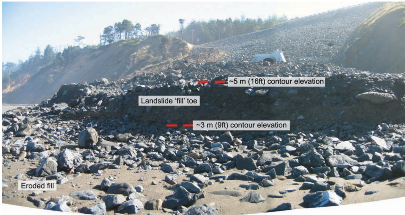
Figure 18. The toe of the artificial landslide on July 14, 2006, showing the presence of an erosion scarp that formed over the latter part of the 2005-2006 winter. To capture the change in position of the landslide toe, various elevation contours (e.g., the 3-m [9 ft] and 5-m [16 ft] contours) are tracked over time. (See Figure 21.)
