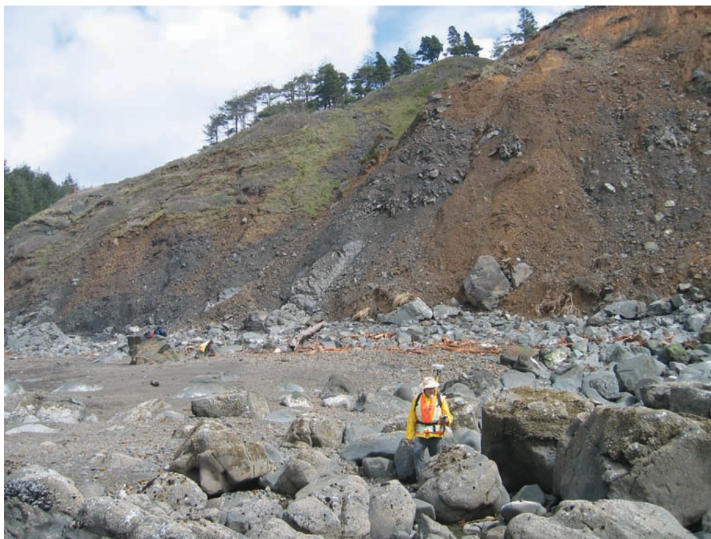
Figure 16. Beach surveys were undertaken by walking lines perpendicular to the water's edge, navigating along a predetermined line identified on a hand-held TSCe Trimble computer connected to the Trimble 5800 GPS rover. The example here is of R. Hart undertaking a topographic survey of the landslide toe adjacent to the Rocky Creek culvert on January 26, 2007. Note the accumulation of gravel associated with the southward transport of some of the fill.
