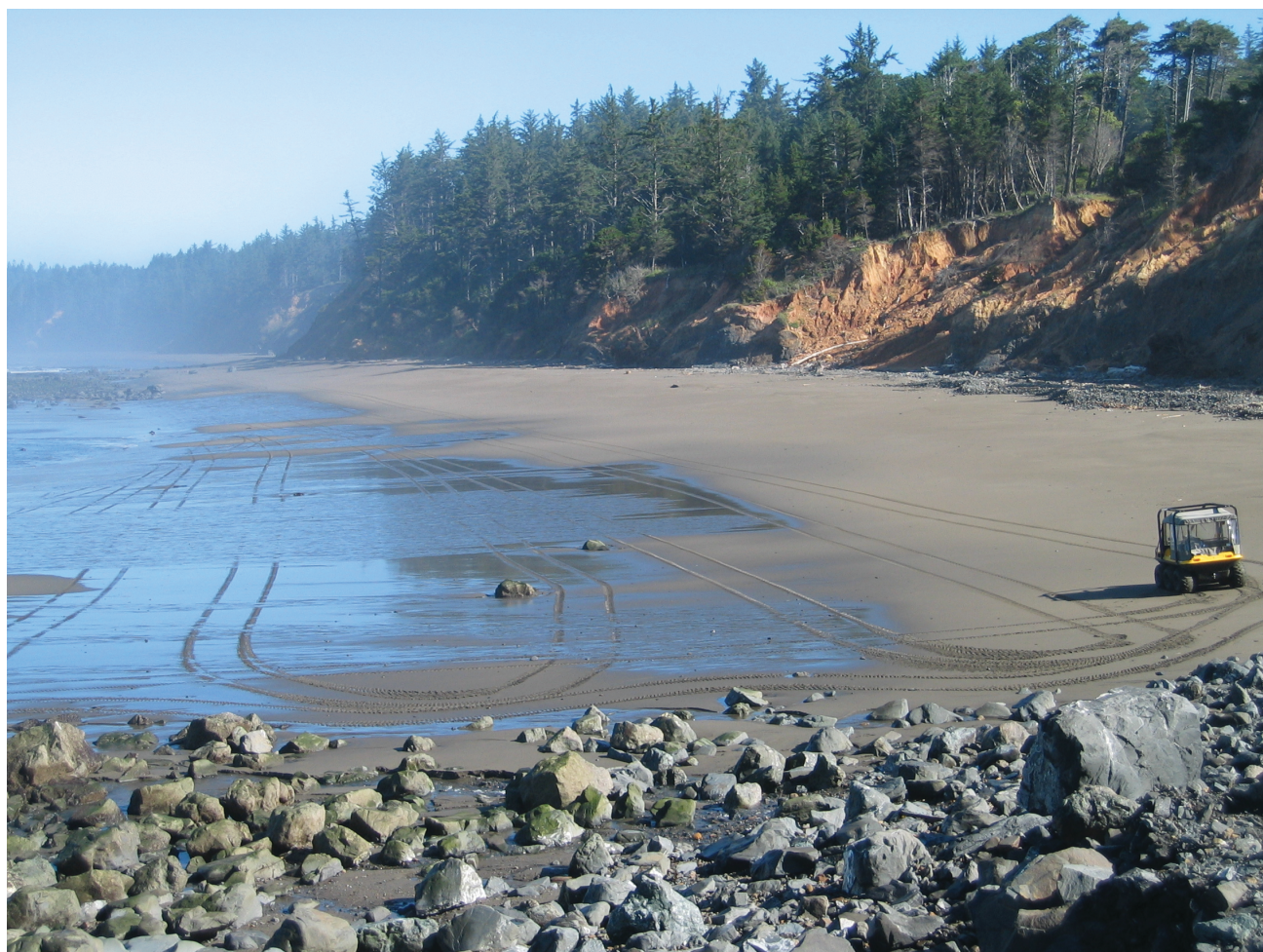
Figure 17. Topographic mapping of the beach was undertaken using a Trimble 5800 GPS unit mounted on top of a six-wheel ARGO ATV. Photo shows the presence of survey tracklines undertaken on the lower beach face, which are spaced roughly 5 to 10 m apart.
