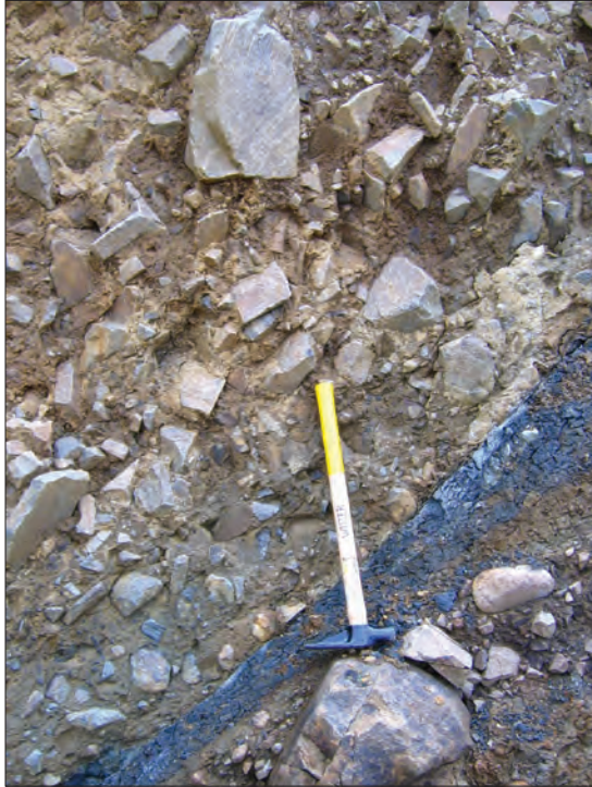
Figure 36. A 10- to 15-cm-thick, dark gray, fat clay gouge layer has developed along the landslide failure plane at the south end of Cove Beach.
