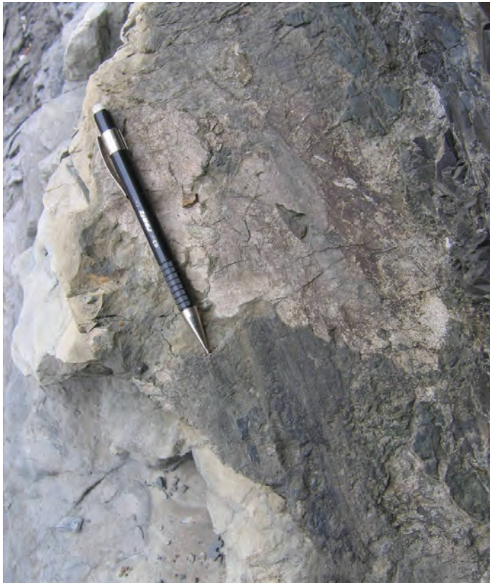
Figure 12. Slip indicators (linear striations parallel to pencil) on a possible landslide failure plane exposed along the beach directly north of the Bald Point, Ecola State Park, indicate a southwest slip direction.
