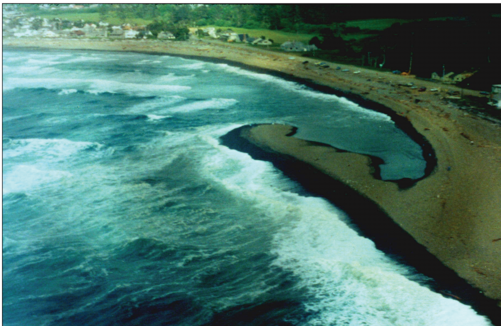
Figure 7. Oblique aerial photo (view to southeast) of a migrating cobble-boulder berm that developed at the cove, at Seaside's southern shoreline, from the 1987 landslide on Tillamook Head. Within one month the berm connected to the north-south beach at the upper left corner of the photo. Larger winter surf pushed the rubble onto the original east-west shoreline (foreground in lower right of photo), killing all intertidal sea life. Waves then moved the cobbles and boulders westward with negligible progradation of the east-west shoreline and onto the north-south beach where the material formed a series of coalescing berms that shifted the shoreline 300 ft westward. The rocky material continues to advance slowly northward along the beach, driven by winter surf. Photo courtesy of Paul D. See.
