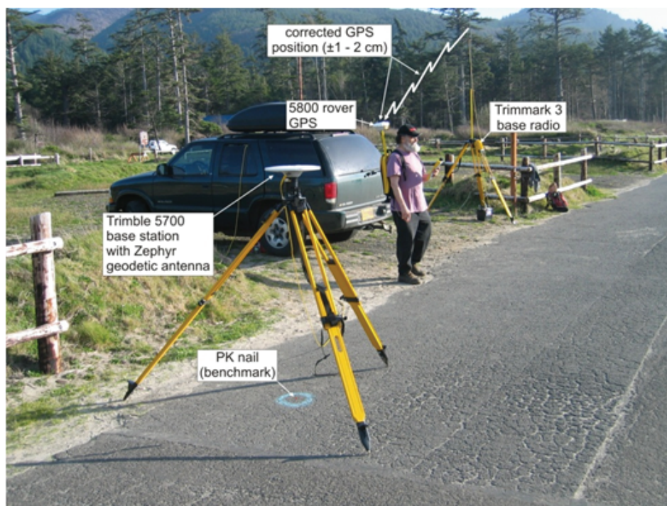
Figure 1. The Trimble 5700 base station antenna located over a known reference point at Cape Lookout State Park. Corrected GPS position and elevation information is then transmitted by a radio modem to the 5800 GPS rover unit.
