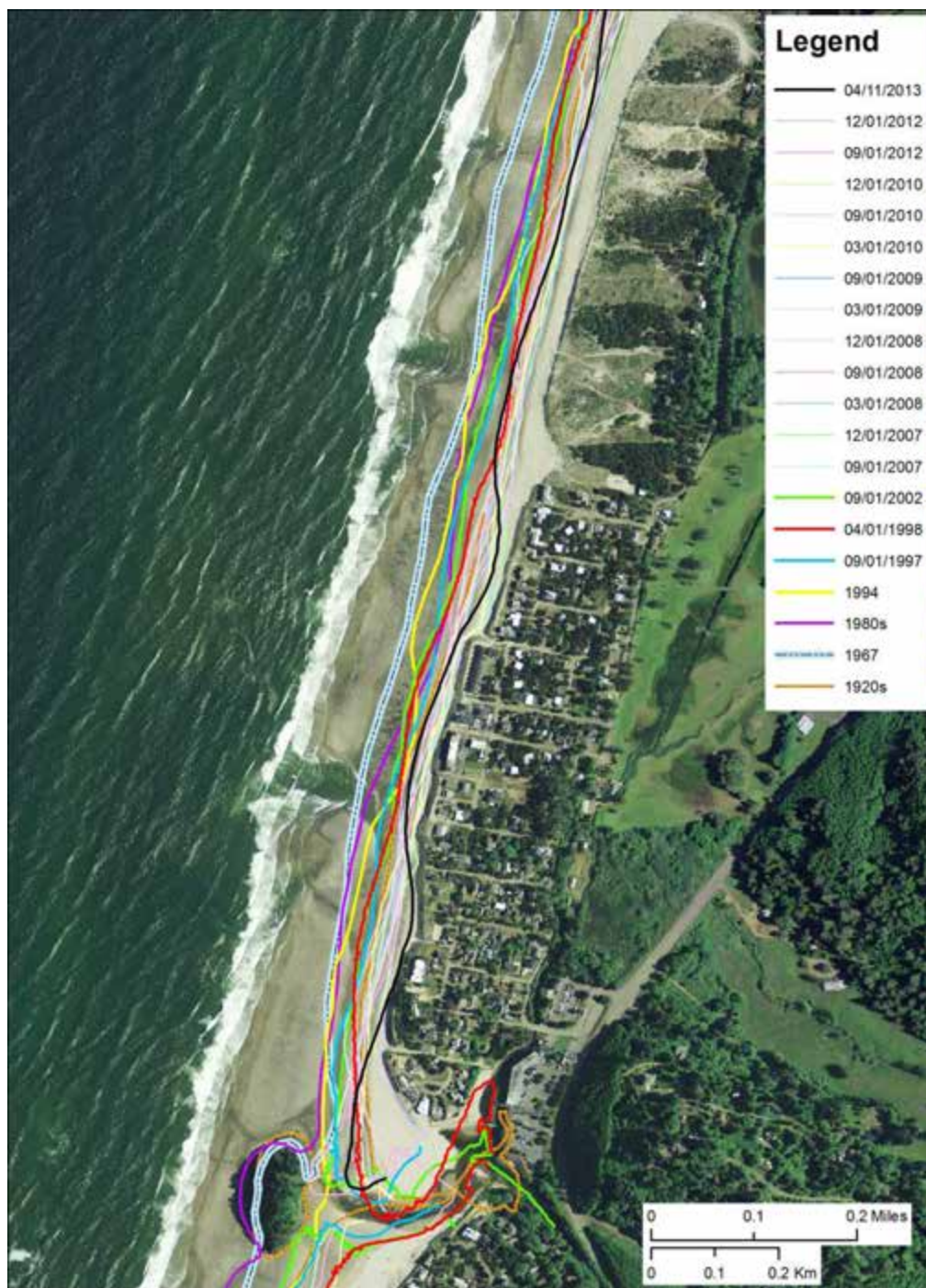
Figure 2-8. Historical and contemporary shoreline positions identified at Neskowin. The 1920s (1927/1928) shoreline is derived from NOST-sheets, 1967 and 1994 shorelines are from orthorectified aerial photographs, 1980s (1985/1986) shorelines are from U.S. Geological Survey topographic maps, 1997–2002 shorelines are derived from lidar, and post 2007 shorelines were measured using GPS.
