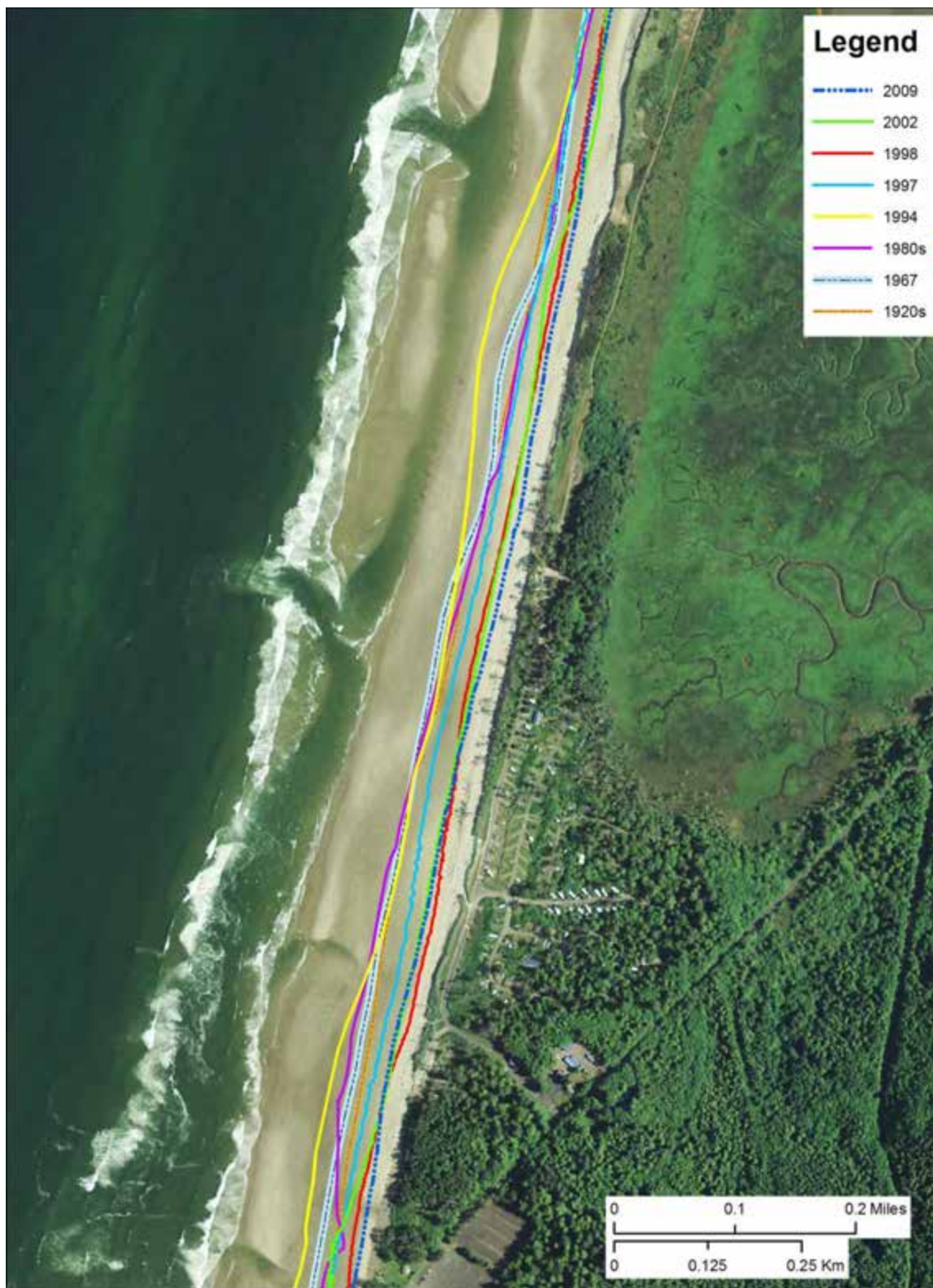
Figure 2-13. Historical and contemporary shoreline positions identified along the southern end of Netarts Spit, adjacent to Cape Lookout State Park. The 1920s (1927/1928) shoreline is derived from NOST-sheets, 1967 and 1994 from orthorectified aerial photographs, 1980s (1985/1986) from U.S. Geological Survey topographic maps, and 1997–2009 are derived from lidar.
