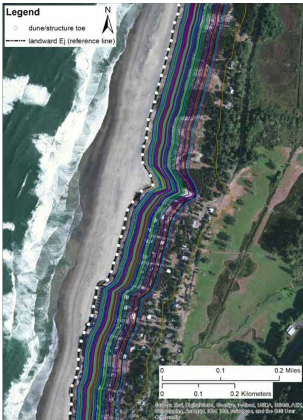
Figure 4-1. Modeled erosion hazard zones for Neskowin showing all 83 scenarios of change (lines). In all cases, the hazard lines are relative to the location of the landward E_j line. White circles depict actual locations of the E_j /structure toe defined from lidar transects spaced 25 m (82 ft) apart.
