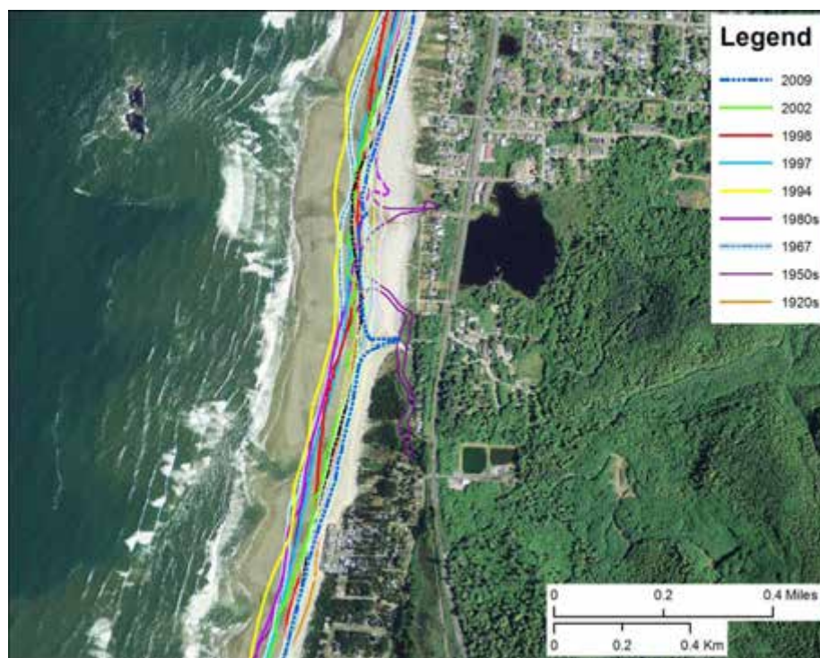
Figure 2-26. Historical shoreline positions identified near Twin Rocks. The 1920s and 1950s (1927/1928, 1953/1955) shoreline is derived from NOS T-sheets, 1967 and 1994 from orthorectified aerial photographs, 1980s (1985/1986) from U.S. Geological Survey topographic maps, and 1997–2009 are derived from lidar.
