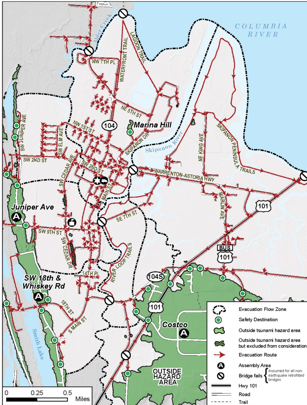
Figure B-1. Least cost (path) distance modeling for the community of Warrenton showing evacuation flow zones and detailed evacuation routes for the scenario assuming all non-retrofitted bridges fail during the earthquake and are unavailable for evacuation.
