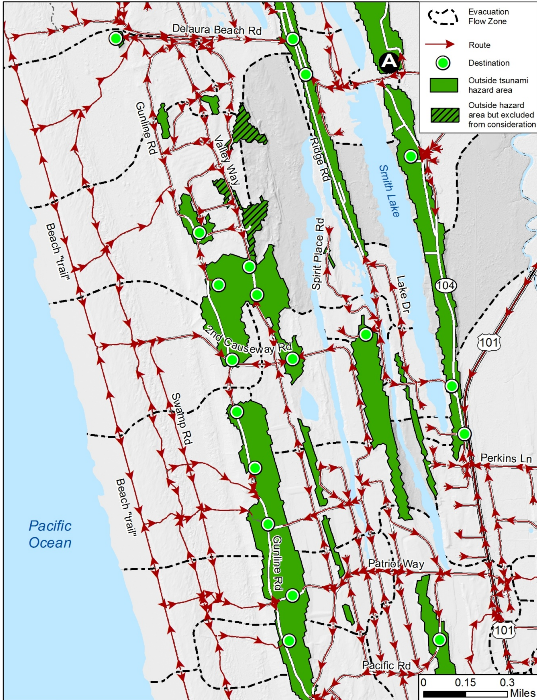
Figure F-1. Least cost (path) distance modeling for Camp Rilea showing evacuation flow zones and detailed evacuation routes.
