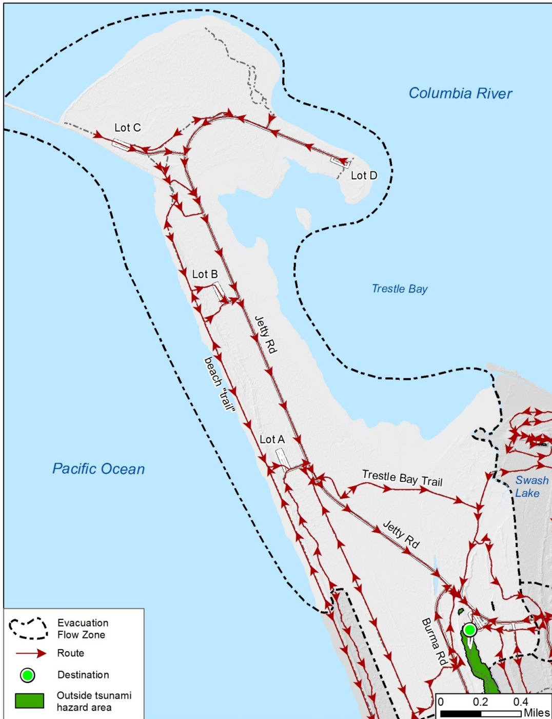
Figure D-1. Least cost (path) distance modeling for the Clatsop Spit showing evacuation flow zones and detailed evacuation routes.
