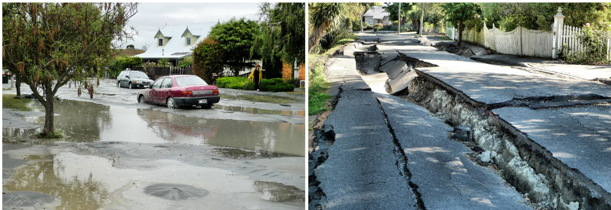
Figure 2-1. Water-saturated sand can turn to quicksand during strong shaking, forming sand boils, ponding, and sunken roads. In these examples, (left) extensive liquefaction occurred along River Road in Christchurch, New Zealand following the February 2011 earthquake, while (right) effects from lateral spreading along numerous Christchurch roads constructed next to waterways resulted in major failures to road infrastructure as roads slumped toward river channels. During a Cascadia subduction zone event, such processes could compromise tsunami evacuation routes as well as the time and speed to safety in areas prone to liquefaction. (Photo credits: Martin Luff, licensed under CC BY-SA 2.0)
