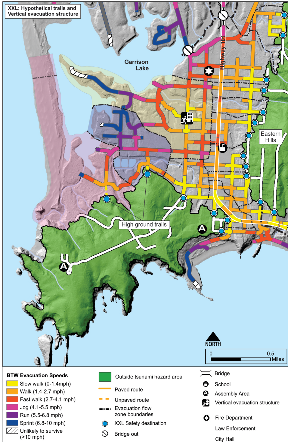
Figure 3-6. Beat the wave tsunami evacuation modeling for Port Orford based on the combined results from a hypothetical tsunami vertical evacuation structure (TVES) and hypothetical southern evacuation trails. Colors on top of the road network reflect BTW minimum travel speeds, while dashed lines define evacuation flow zone boundaries. The pink and blue shaded regions define the area that would be served by the proposed hypothetical trails; the yellow region defines the TVES evacuation flow zone. Highway 101 is highlighted in white to emphasize the divide between evacuating east to the foothills and west to the hypothetical TVES.
