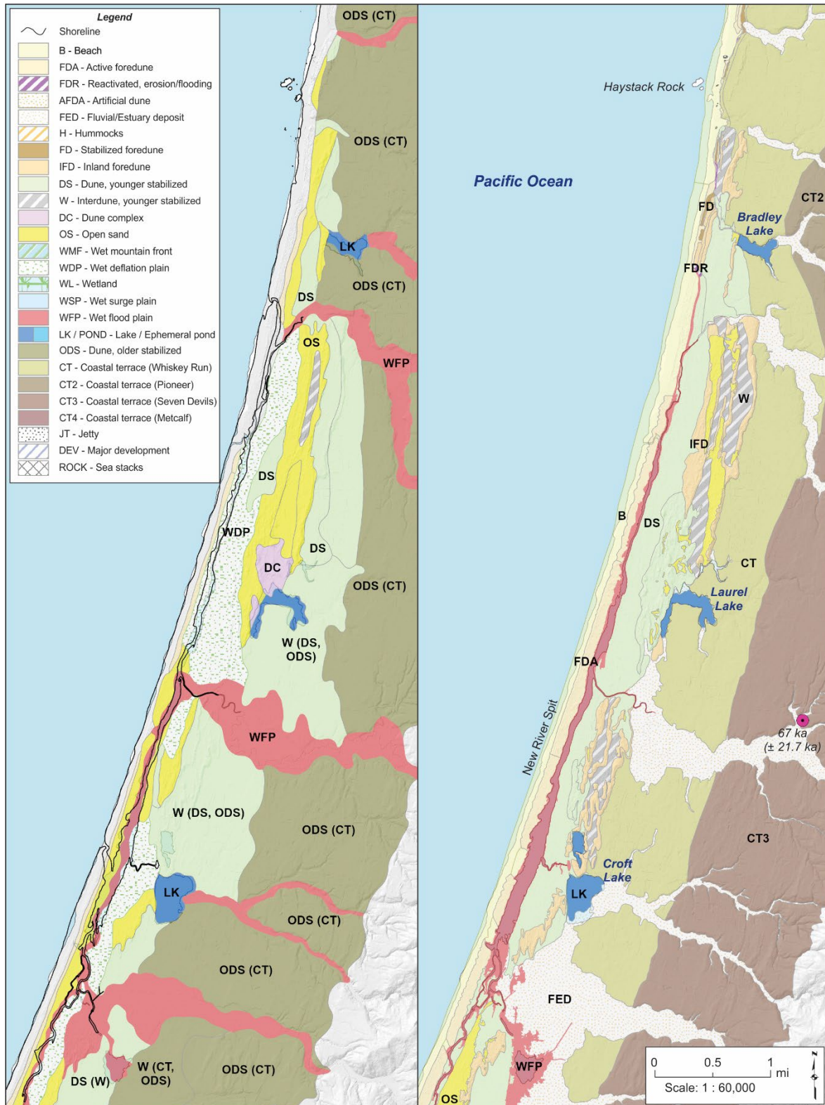
Figure 4.3. Beach and dune geomorphic mapping classifications for the New River Spit. (left) original USDA (1975), (right) updated version. Green and pink circles, respectively, denote ^{14}\text{C} and thermoluminescence (TL) dates determined by Peterson and others (2007).
