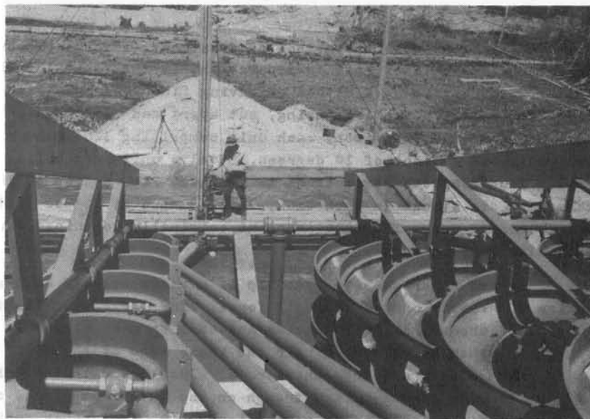
TOP VIEW OF HUMPHREYS SPIRAL CONCENTRATORS.
