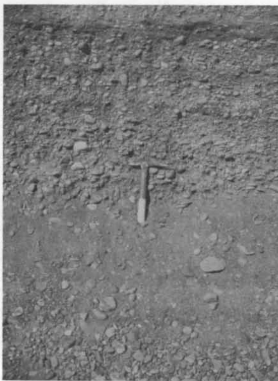
Fig.4. Typical Willamette River flood-plain deposits in the channel-belt area. Note the absence of cemented layers and the relatively greater amount of fine-grained (sand) matrix.
