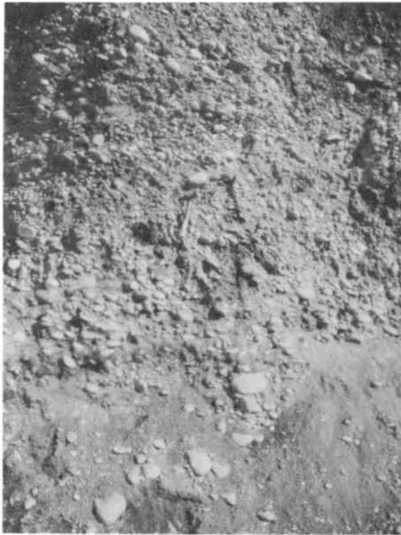
Fig.5. Typical Salem-Santiam fan deposits at the Walling Sand & Gravel operation. The pick head is approximately 2 feet below the upper weathered zone.
