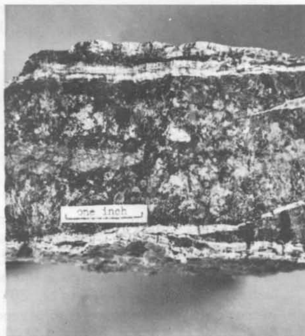
Cross-fibre chrysotile veinlets in serpentine from the Foster asbestos deposit near Josephine Creek. Samples were selected from the dump of the southern adit.
