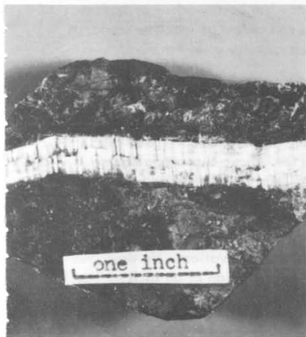
Cross-fibre chrysotile veinlets in serpentine from the Foster asbestos deposit near Josephine Creek. Samples were selected from the dump of the southern adit.
