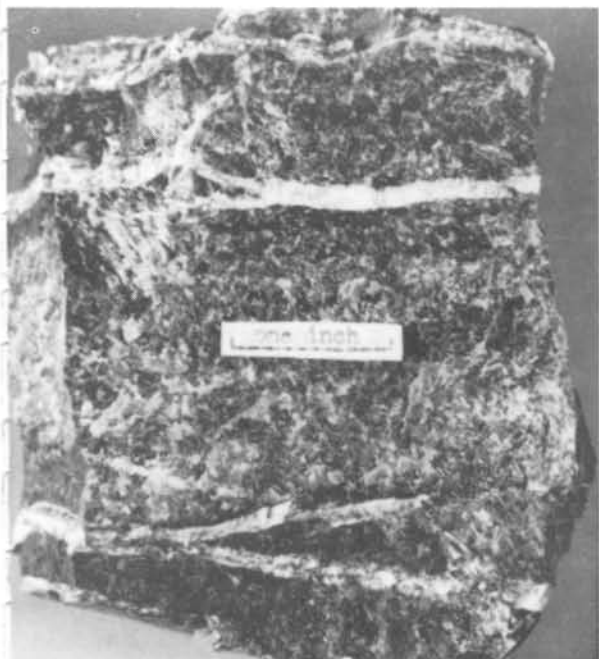
Cross-fibre chrysotile veinlets in serpentine from the Foster asbestos deposit near Josephine Creek. Samples were selected from the dump of the southern adit.
