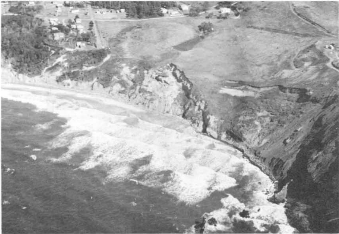
Figure 9. Slumping of Astoria Formation and overlying terrace deposits adjacent to north side of Yaquina Head.
