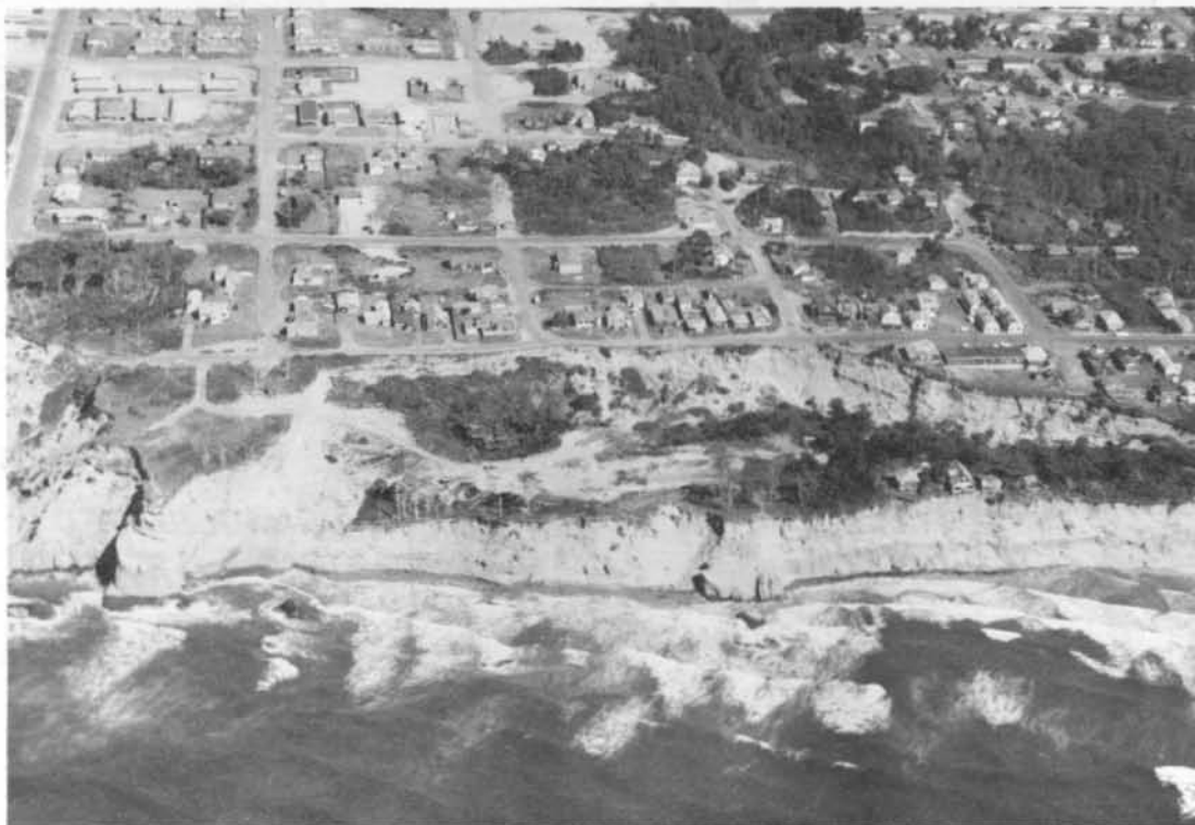
Figure 10. Terrace slump in an area of seaward-dipping Miocene sandstones and shales at Newport.
