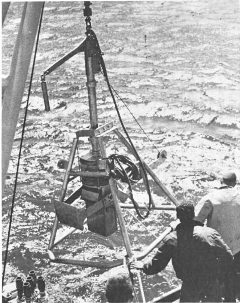
Figure 3. Box corer. After the corer has penetrated the sediment, the large knife cuts through the sediment closing off the bottom of the rectangular box.
