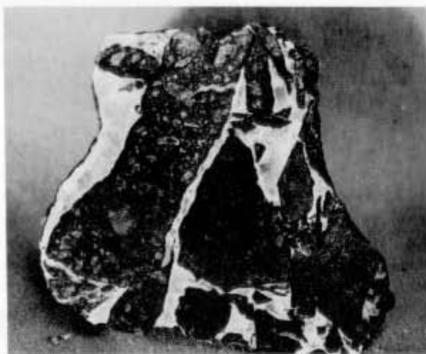
Figure 5. A cut section of rock from the brecciated zone at Coburg Butte showing cementation by thompsonite and analcime. X0.7
