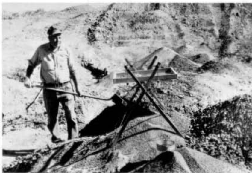
Figure 10. A typical sunstone mining operation. The thin overburden has been removed exposing decomposed basalt, which is easily disintegrated by hand picks and chisels and then screened to separate the sunstones.
