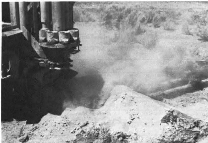
Close-up of air drill showing the automatic pipe-handling rack. Rubber skirts catch and hold cuttings around bore hole.
