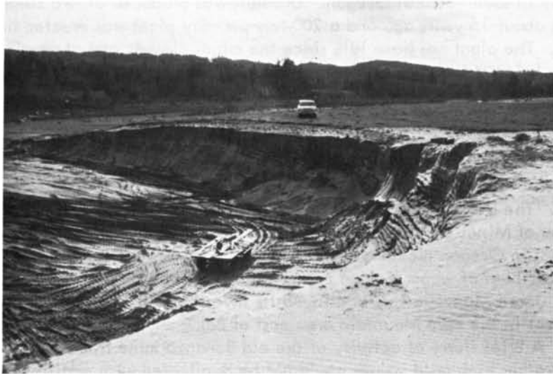
A sand deposit in Clatsop County undergoes concurrent excavation and reclamation. Area of removal is limited to 2 acres; that beyond the pit has already been reclaimed.
