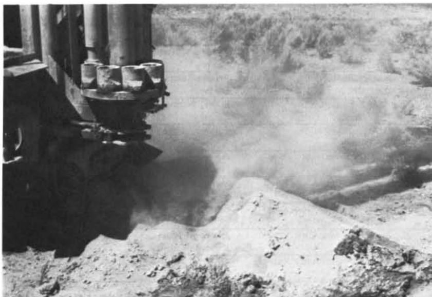
Close-up of air drill showing the automatic pipe-handling rack. Rubber skirts catch and hold cuttings around bore hole.
