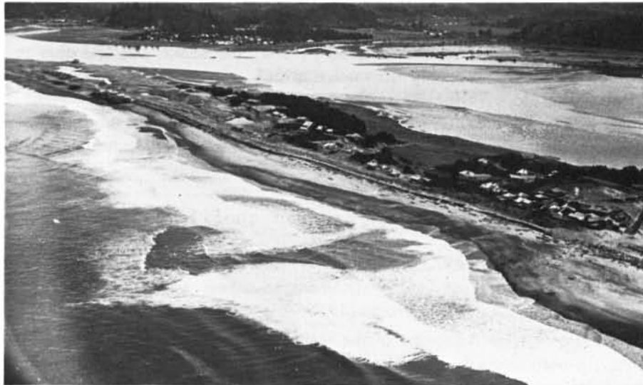
Figure 8. Irregular shoreline of bays and cusps are due to rip currents, one of which is shown in this photograph taken February 8, 1973.
