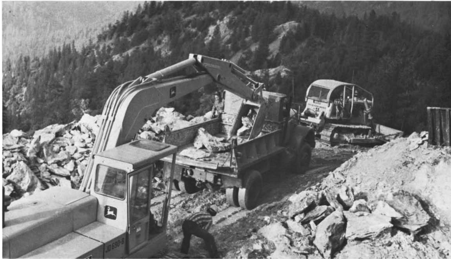
Figure 7. Soapstone blocks are removed and loaded with large backhoe and smaller front-end loaders for haulage to Dividend Bar, where they are stockpiled.
