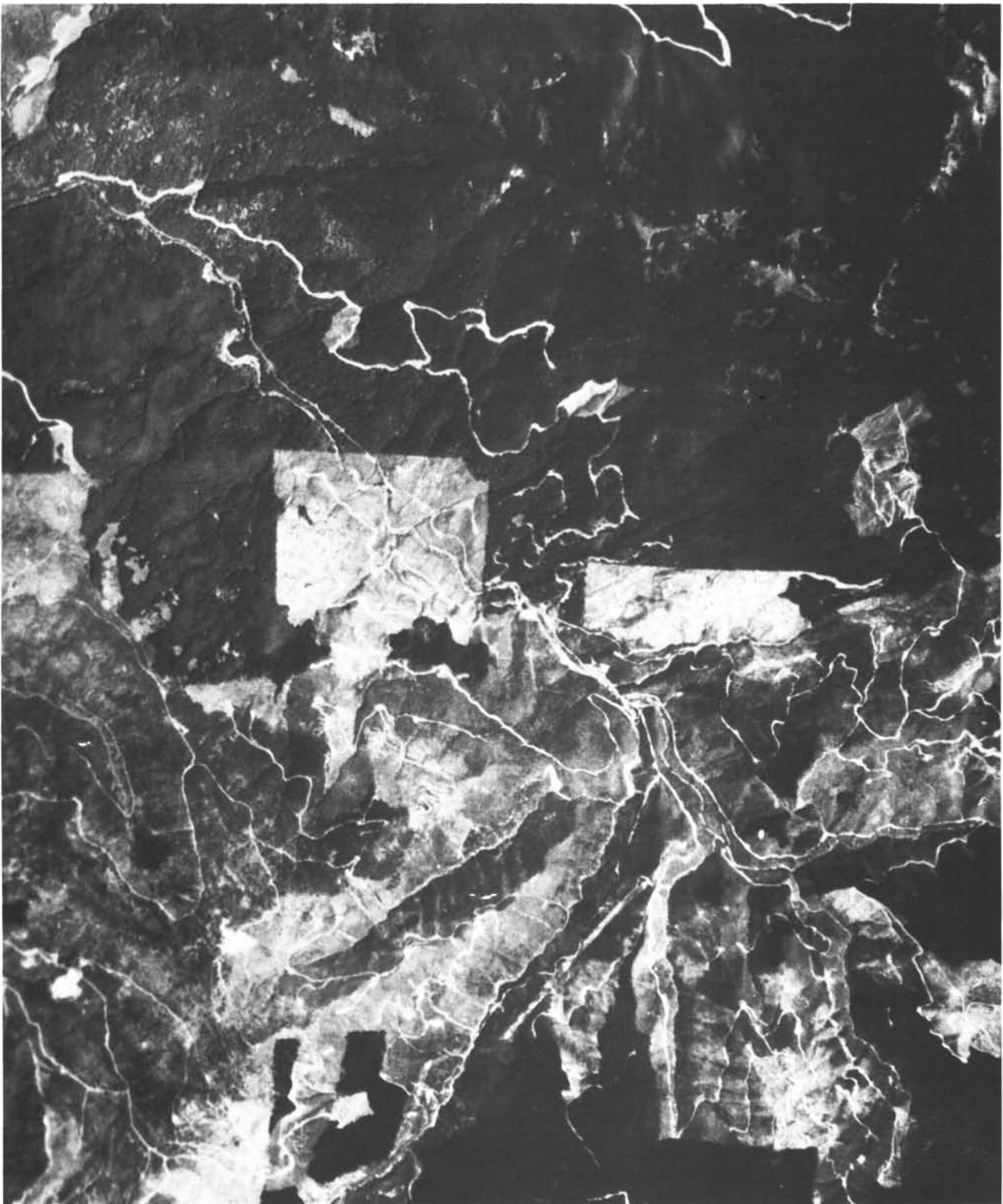
Figure 9. Example of NASA high-altitude imagery of upper Molalla River Basin. By using stereo and high magnification, one can distinguish such erosional features as slump/earthflows, debris avalanches, talus, road failures, stream-bank failures, mining excavations, and large gullies; depositional features such as streambed deposits and debris jams; and various land management methods and practices. Lighter areas represent recent clear-cut harvesting, while darker areas show old-growth timber. (Photo courtesy National Aeronautics and Space Administration)
