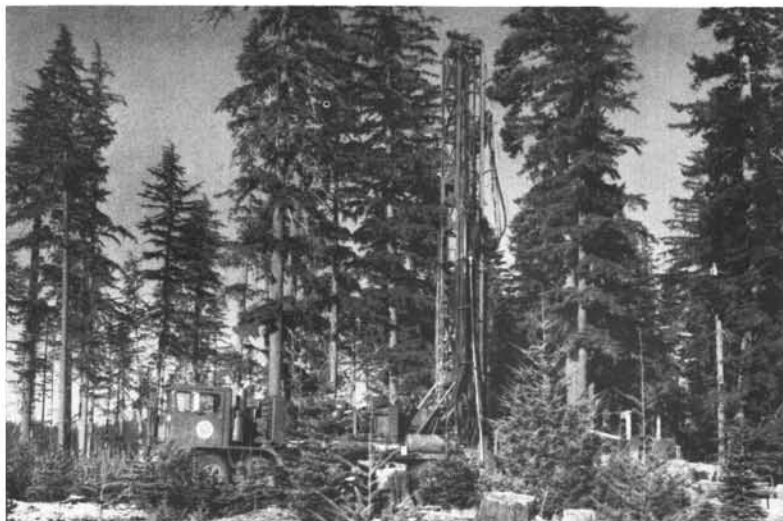
Figure 5. Thermal gradient drilling by Oregon Department of Geology and Mineral Industries near Clear Lake, Wasco County, November, 1978.
