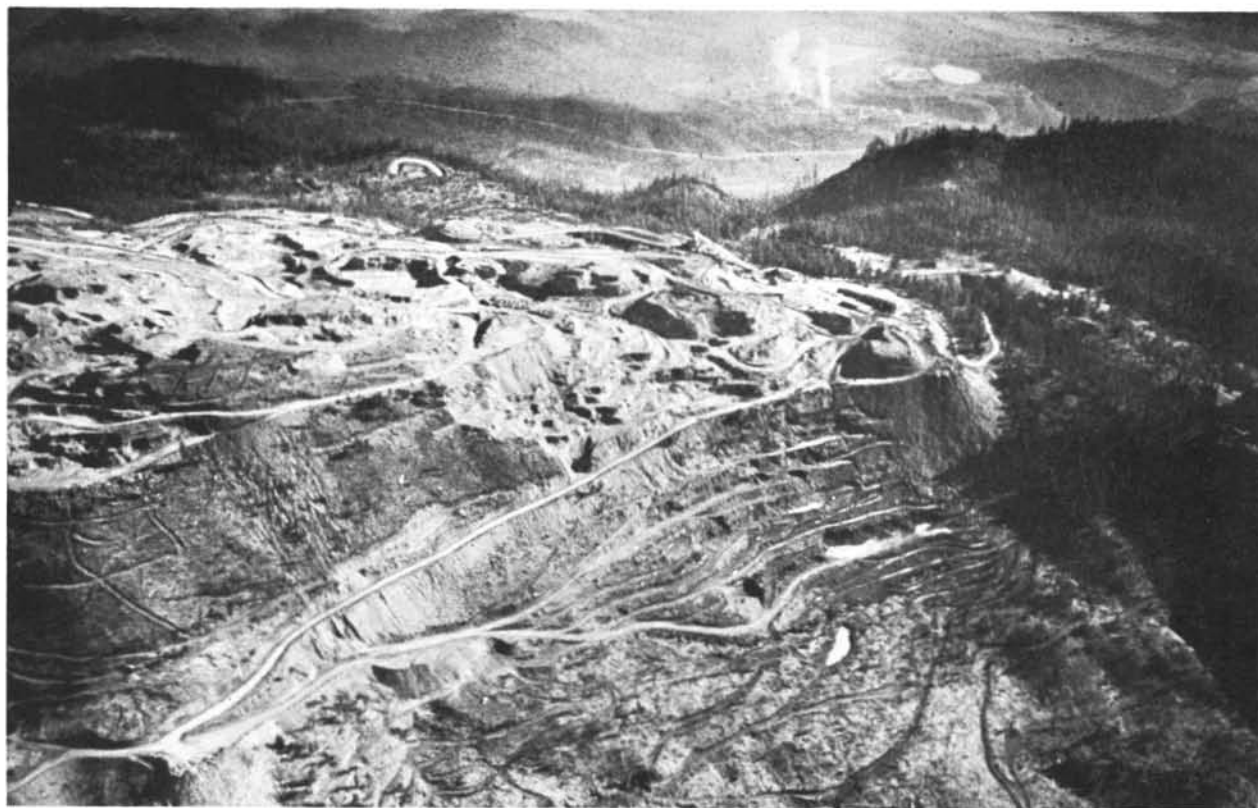
Figure 4. Nickel Mountain, site of only active nickel mine in United States, located near town of Riddle, Douglas County. Smelter located in background and mine employ about 580 people and annually produce ferronickel worth approximately $50 million.
