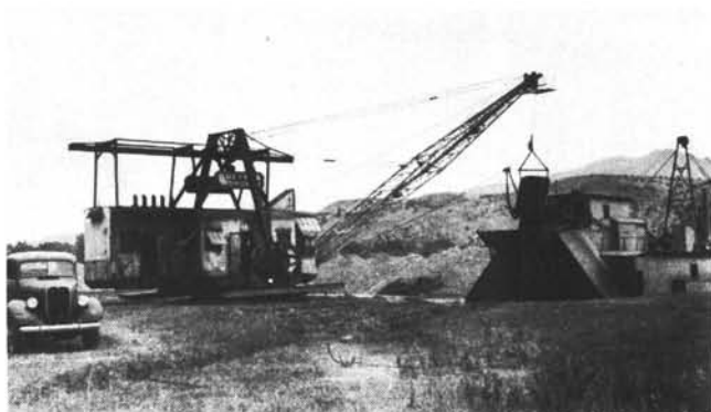
Ferris and Marchbank operation, showing dragline and floating washing plant.
