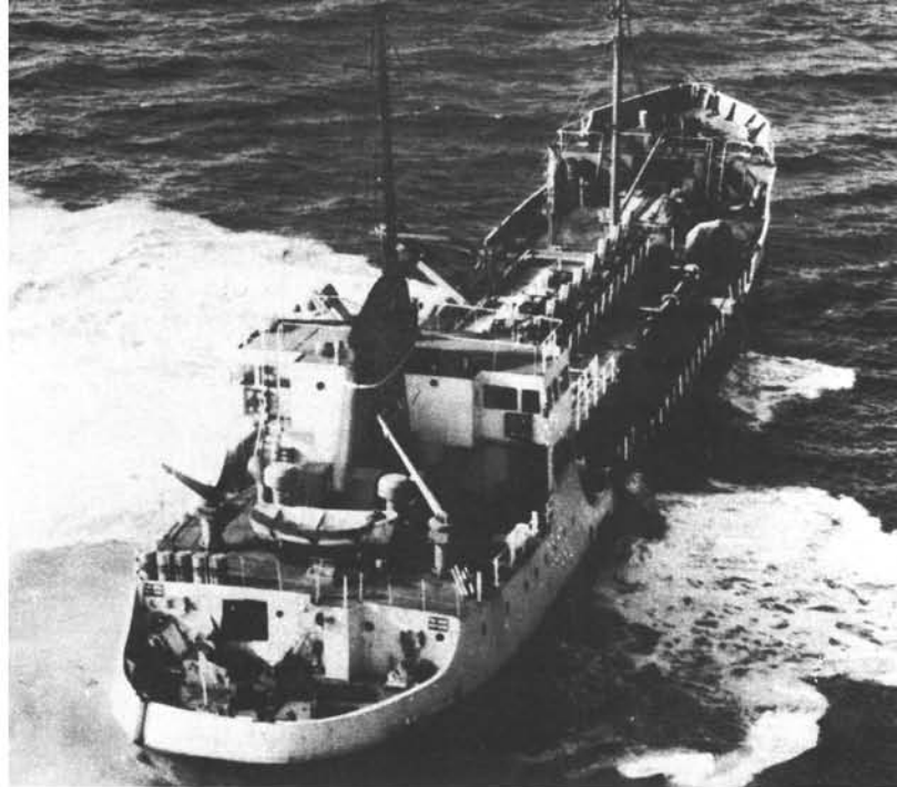
Figure 1. British sand and gravel dredger Cambrook, built in 1967, has capacity of well over 2,000 tons. (Photo from Hess, 1971)
