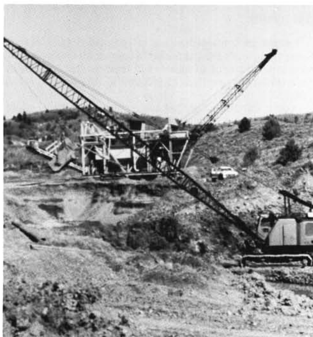
Ground level view of Mormon Basin Placer, Inc., gold placer operation on Basin Creek, showing draglines and gold recovery plant.
