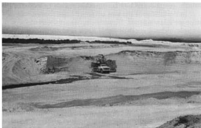
Figure 3. Oil-Dri pit, looking north. Diatomite is quarried along pervasive north-south joint set. OD section was measured at south end of pit, just to left of photograph.
