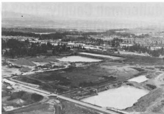
Excavation starting in 1980 on former mining-landfill site in preparation for Multnomah County's new operation and maintenance headquarters (center). Note continuing mining-related activities on all sides. (State Highway Division air photo)
