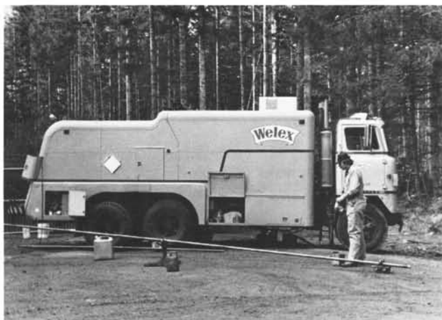
Welex personnel preparing to run a bridge plug to stop water production at Reichhold Columbia County 4 at Mist Gas Field.
