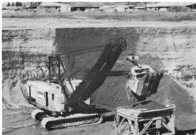
Bringing sand and gravel up from a deposit near the confluence of the McKenzie and Willamette Rivers with a shovel-and-conveyor belt system. (Photo courtesy Wildish Sand and Gravel Co.)
