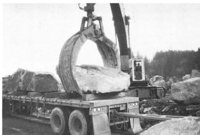
Jettystone is loaded at the quarry of Kiewit Pacific Company near Mapleton in Lane County. The stone will be used in extending jetties at the mouth of the Siuslaw River.
