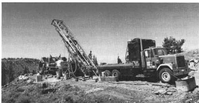
Reverse circulation drilling on American Copper and Nickel Company property in the Sunrise Butte area of Grant County.
