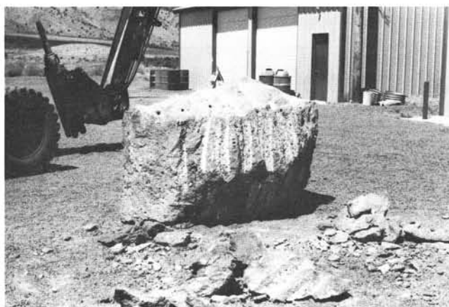
Final shape of the basalt rock before it was crated up for shipment. Note vertical stripes from hydraulic impact hammer.
