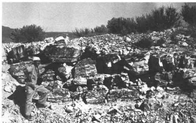
Figure 3. Clinoptilolite-rich tuff exposed in a bulldozer cut at the Sheaville, Oregon, zeolite deposit at the stop described in Part A of this paper. Bedding dips northwestward (to the left). The moderately resistant tuff breaks with a hackly to subconchoidal fracture.
