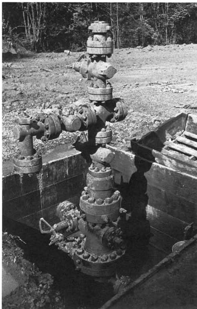
Wellhead at the ARCO Columbia County 31-27-65, which was drilled to a total depth of 6,700 ft, making it the deepest well drilled during 1987.
