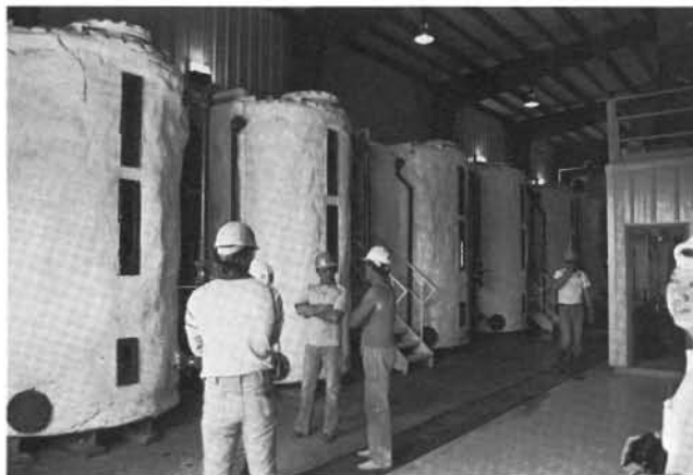
Example of carbon columns used to remove gold from pregnant solution.
