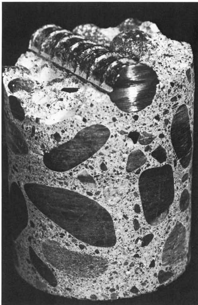
Figure 13. Columnar section of rebar concrete taken from a building foundation. Samples such as this are extracted from building foundations and tested to ensure that the rebar and concrete are sound. Note how the cement-and-water paste completely coats each aggregate particle. Photo by David Parke.
