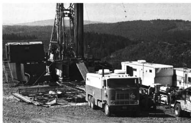
Logging operations at well IW 42C-10 of Oregon Natural Gas Development Company as part of the natural-gas storage project at Mist Gas Field.
