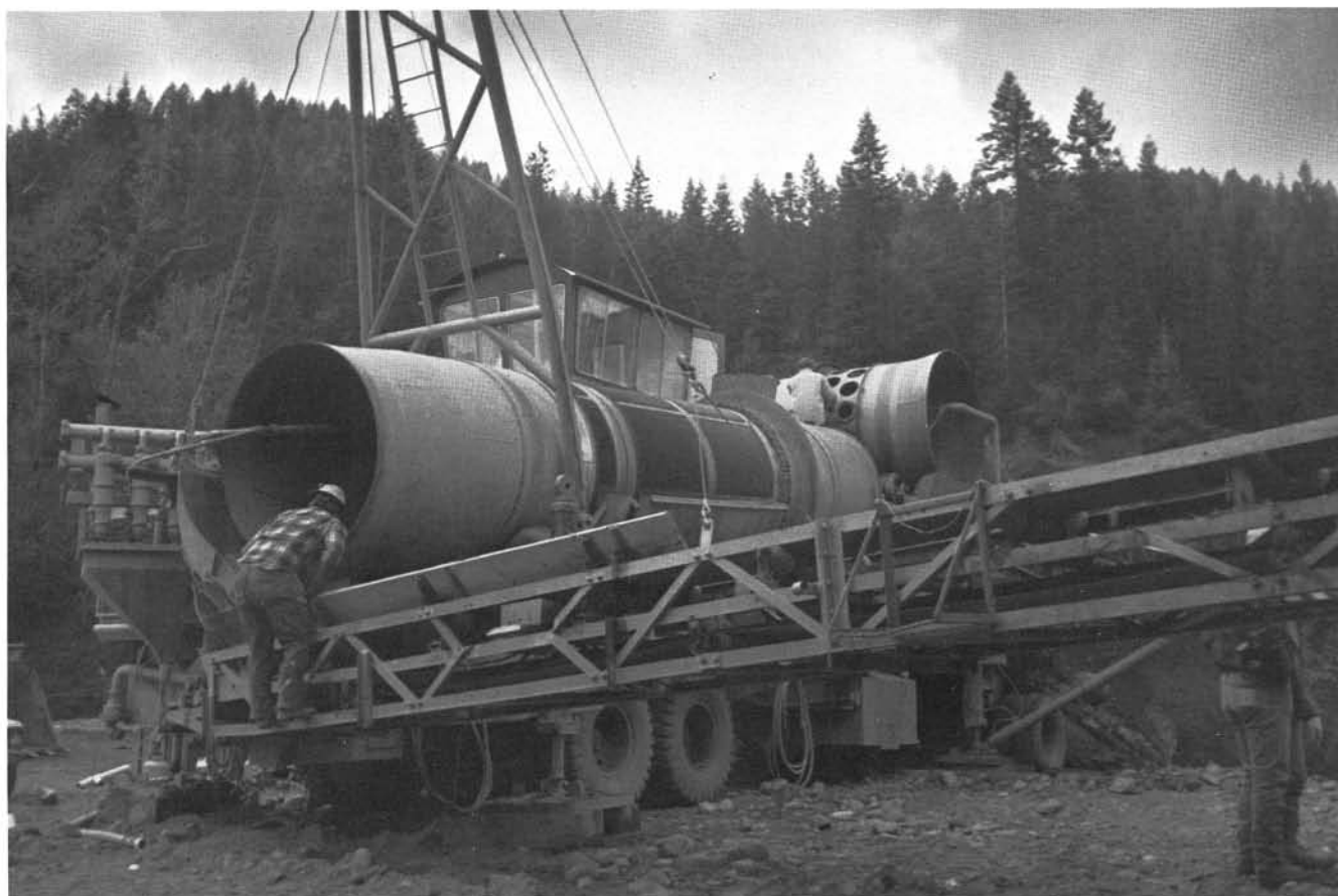
Dry-land dredge plant in operation at Bonanza Mine (active mine site 7) in Baker County.
