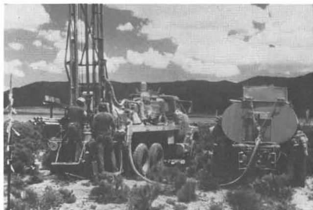
A shot hole is drilled, and an explosive charge is buried and later detonated to create a seismic sound charge.
