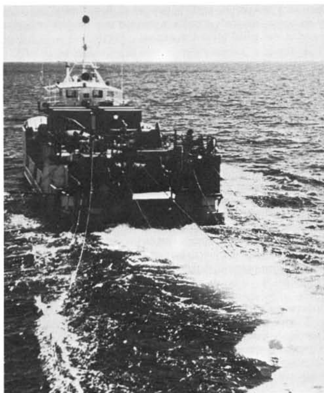
Marine geophysical vessel towing (1) air guns that release compressed air to generate pressure impulses, and (2) hydrophones that receive the reflected signal generated by the air guns.
