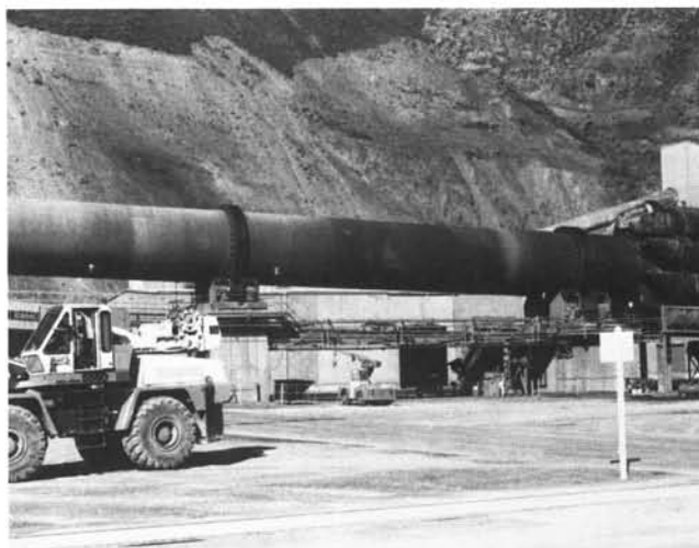
The 216-ft, gas/coal-fired rotary kiln at Ash Grove Cement West in Durkee. Ground limestone and shale are fed in from the left, fused to clinker in the central 2,700 °F-hot zone, and the clinker is cooled and discharged at the right.
