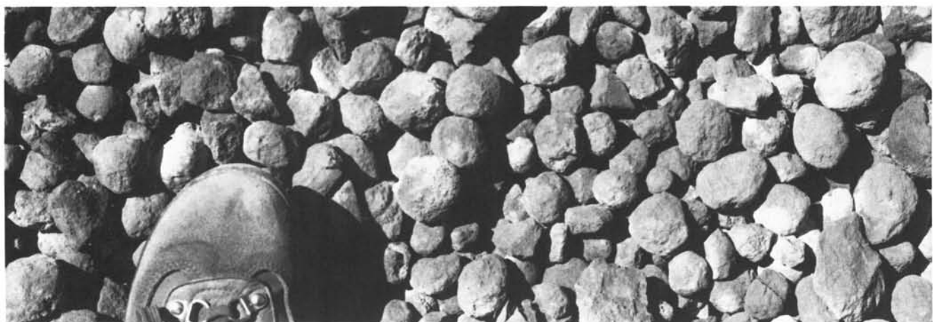
Clinker from the rotary kiln at Ash Grove Cement West in Durkee. It is subsequently ground to a fine powder and blended with gypsum to make portland cement.
