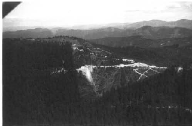
Figure 3. Formosa Resources' Silver Peak Mine (Mine site 23, Table 2) is producing copper, zinc, silver, and gold. Mill and settling pond are located on the ridge crest, and ore is trucked to the mill from the portal at left.
