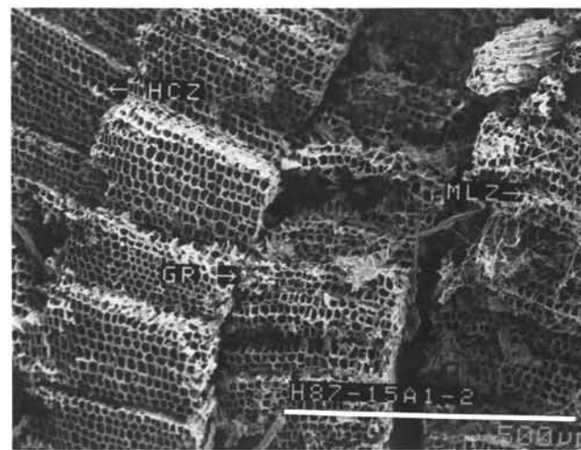
Figure 5. Sample of partially carbonized wood from the Mount St. Helens blast deposit, showing a homogenized-cell zone (HCZ), a zone with middle lamellae still present (MLZ), and the curvature of growth rings (GR) (Sample H87-15A1-2). Bar = 500 \mu .
