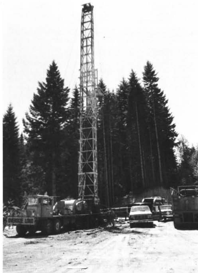
Figure 1. Preparations to flow test the Nahama and Weagant Energy well CC 43-33-75. Flow tests are done on all successful gas wells to determine the amount of gas the well is capable of producing and to measure reservoir pressures in the well.
