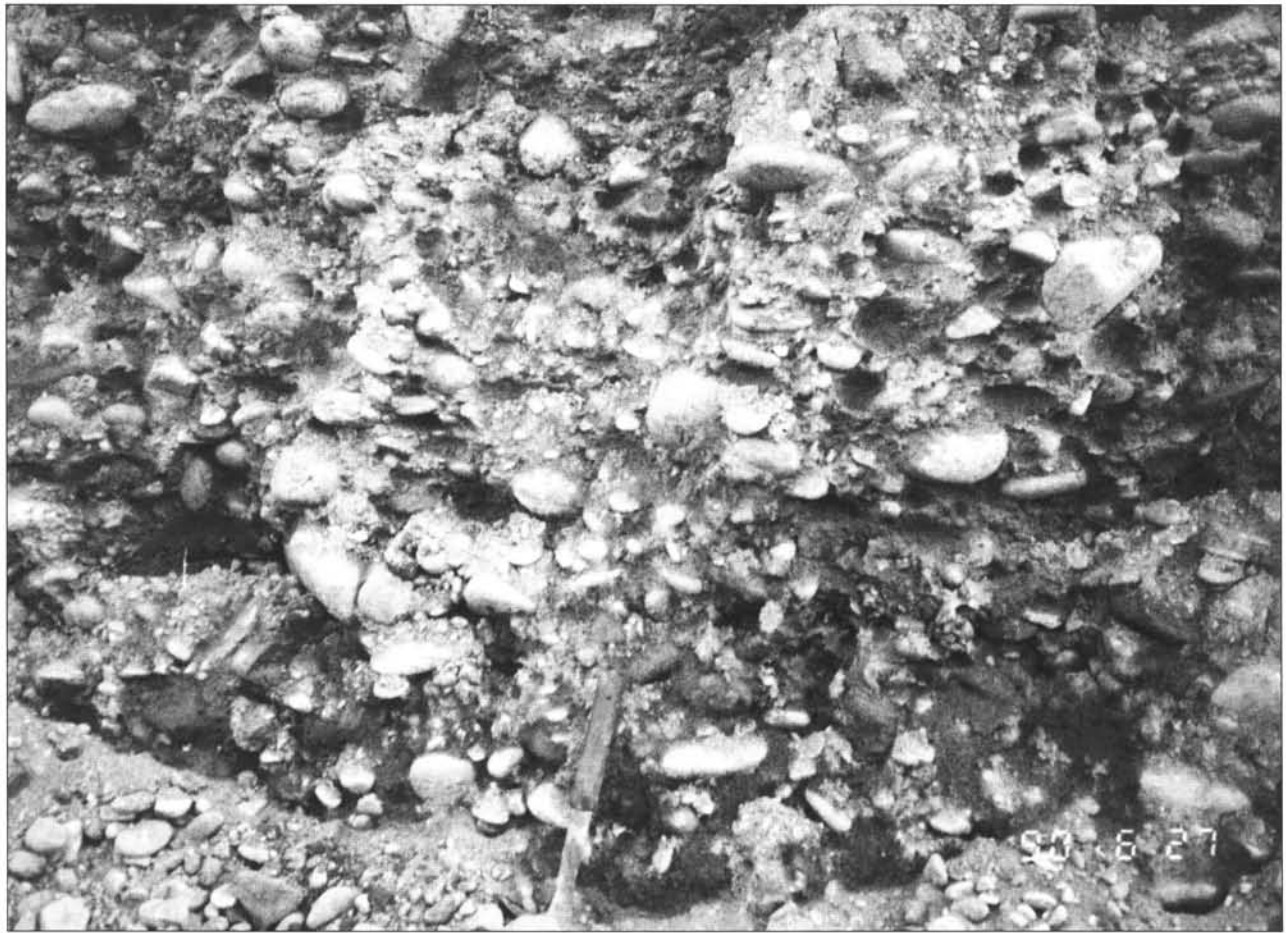
Figure 7. Unconformable contacts exposed during construction activities along NE Sandy Boulevard (see Figure 2 for location). Lower contact is the angular unconformity between Pleistocene gravel unit 2 and the underlying Troutdale Formation. Unit designations are the same as in Figure 5.
