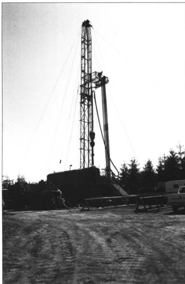
Drilling operation at the Nahama and Weagant well LF 43-32-65, which was drilled by Taylor Drilling Company Rig 7 and was completed as a gas producer during 1993 at the Mist Gas Field. The well produced gas at a rate of over 2 million cubic feet per day during its first month of production.
