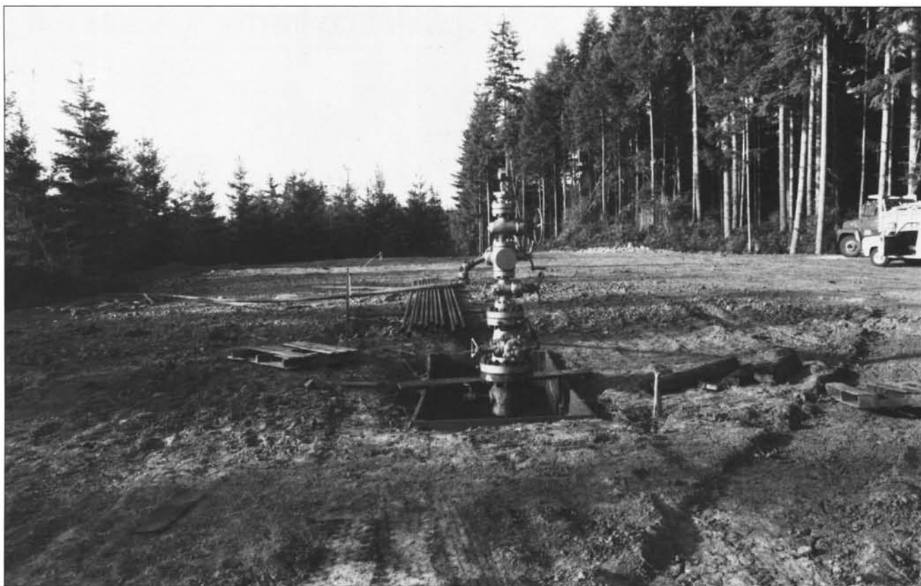
Wellhead at the LF 31-36-65 well, which was operated by Nahama and Weagant and completed as a gas producer during 1993 at the Mist Gas Field.
